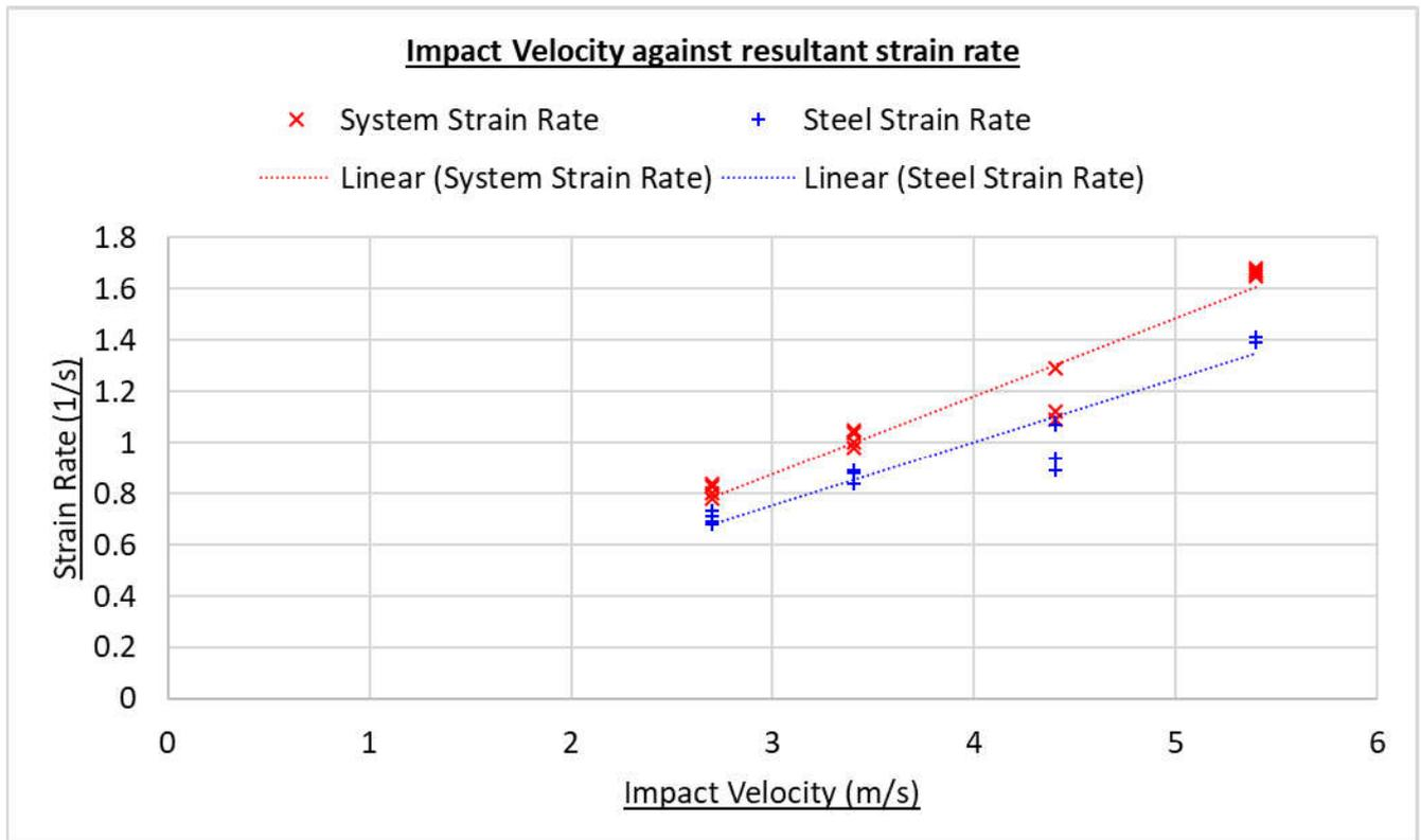
FIG 7 – The correlation between the impact velocity and the strain rate for the first impulse of each sample
